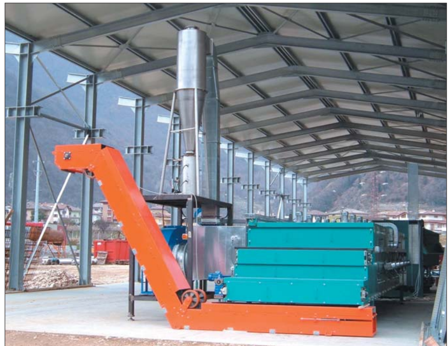
Siemens' new convective Sludge Belt Dryer offers such system advantages as efficient operation in minimal space, low emissions, low dust, a granular final product, and a low thermal requirement with possible heat recovery from low temperature waste energy sources.
