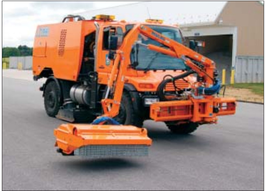
The front-mount boom mower from Mulag on York Township's Unimog comes in handy for roadside maintenance operations.
