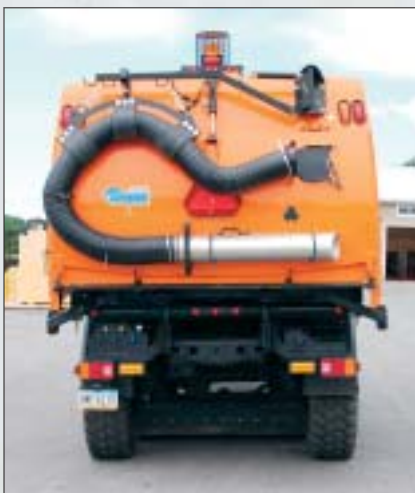
York Township's Unimog includes a regenerative air sweeper.
