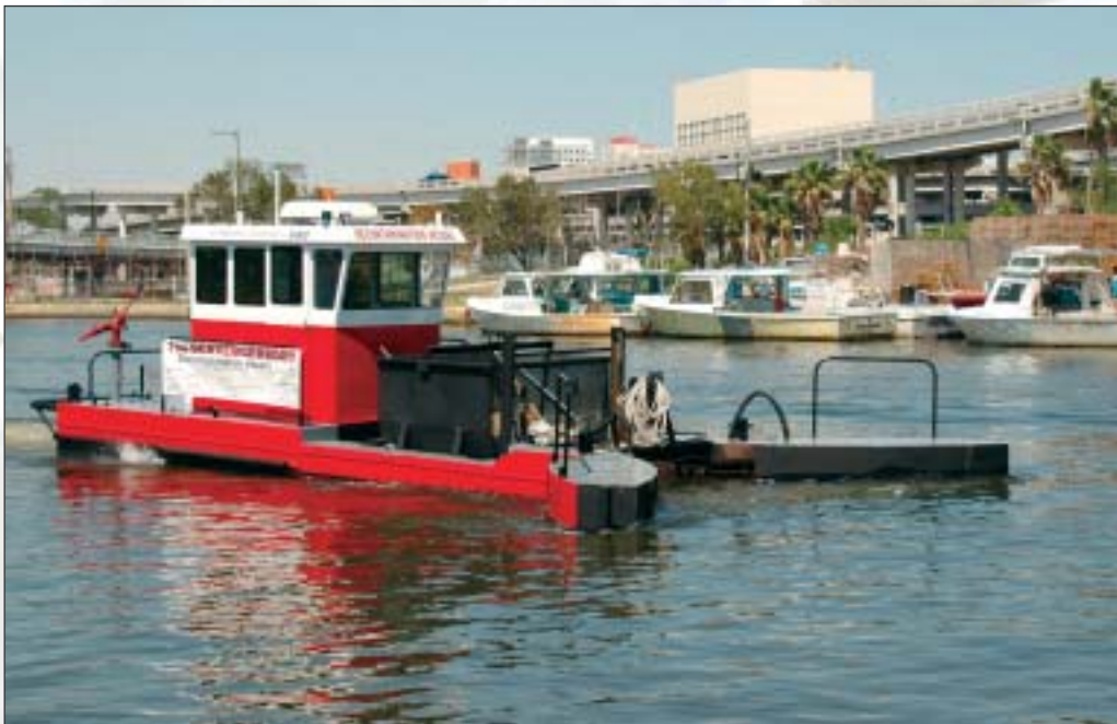
Scavenger has a narrow beam—only eight feet—but opens its split bow from the center, mimicking the claw of a lobster, to dramatically widen its sweep through the Miami River.
