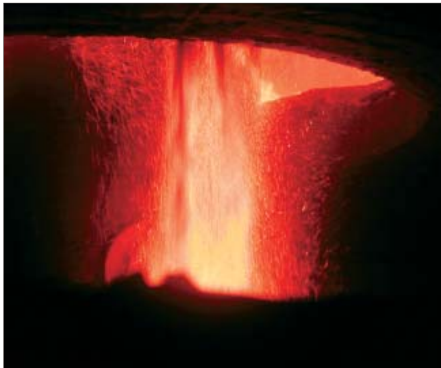
Burning sludge and ash cascade from hearth to hearth at the GBMSD facility. (Photo credit: Incinerator Rx)
