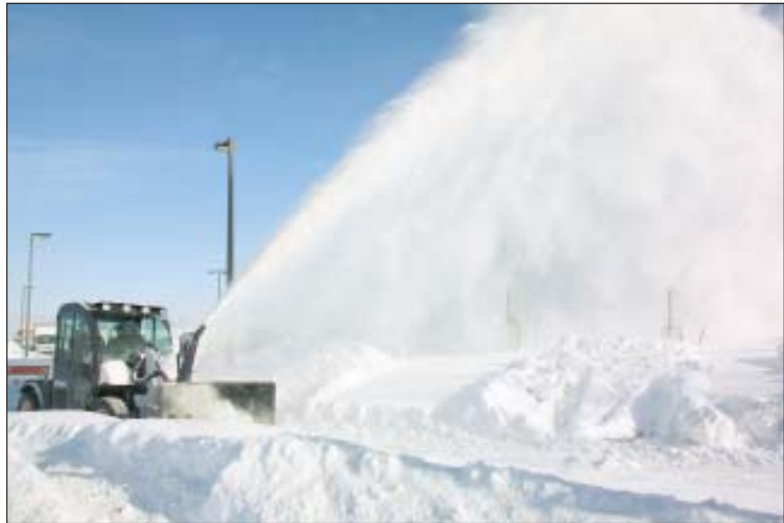
Snowblower attachments on utility work machines facilitate snow removal off sidewalks or in tight places where only a small machine can fit.
