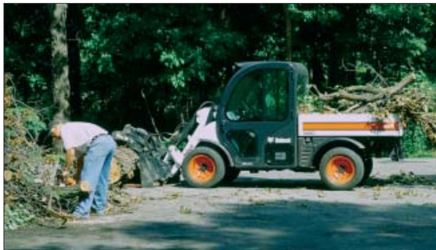
Forks and grapples hitched to a utility work machine help make short work of cleaning up trees and branches.
