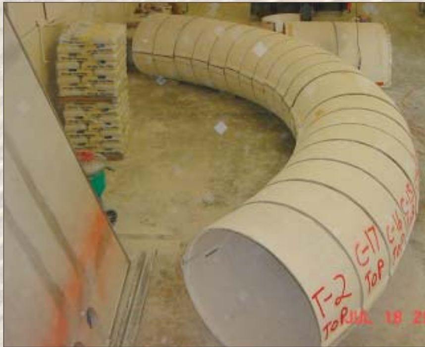
This test assembly of the 90-degree bend was first done on the manufacturing plant floor to verify the proper alignment.
