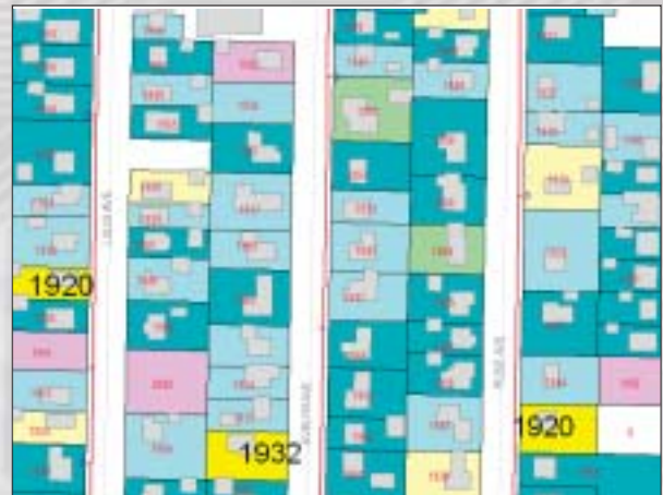
Figure 3. Finding the oldest building structures to estimate the age of the infrastructure.
