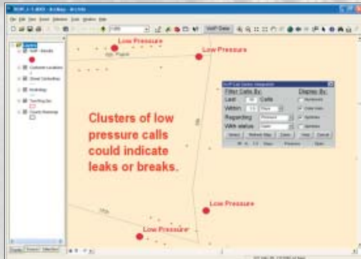
Figure 5. Call Center GIS display of four low pressure calls on different streets.
