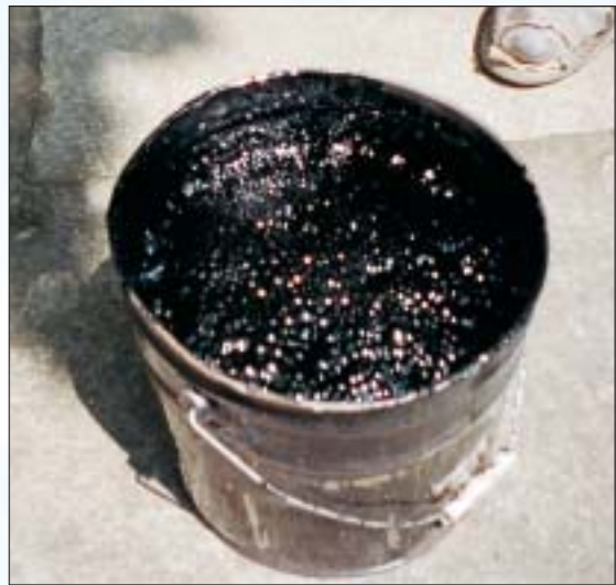
Bucket holds the hot foamed asphalt shortly after it has been extracted from the sample nozzle on the pulverizer. Typically the asphalt cement is expanded 10 to 12 times its normal volume.
