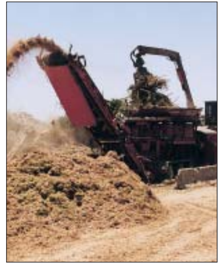
Having a pair of tub grinders now allows some auxiliary grinding in the area.
