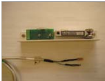
Wireless tilt sensors are attached to the Tobin Memorial Bridge, providing data that will be calibrated against actual conditions.
