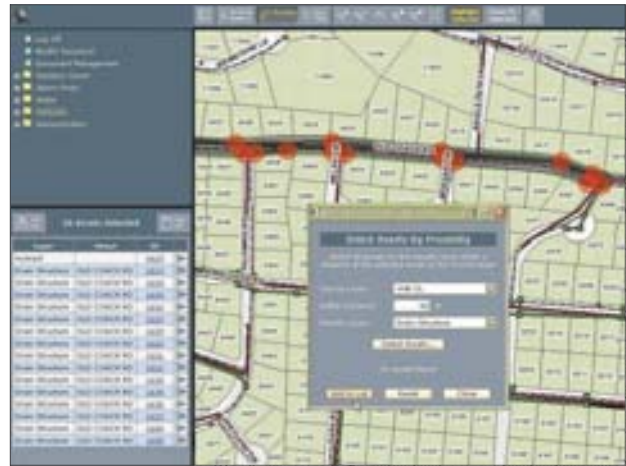
The Proximity Command enables users to select all assets on the Results layer within a distance of the selected asset on the Source layer.
