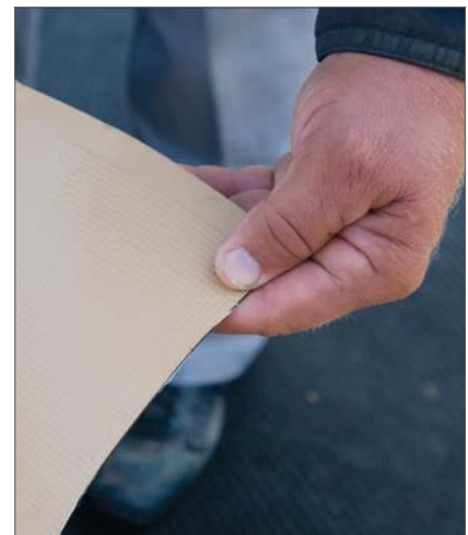
High-performance 65 mil five-ply liner is leakproof, stabilizes the soil, and has an expected service life of at least 25 years.
