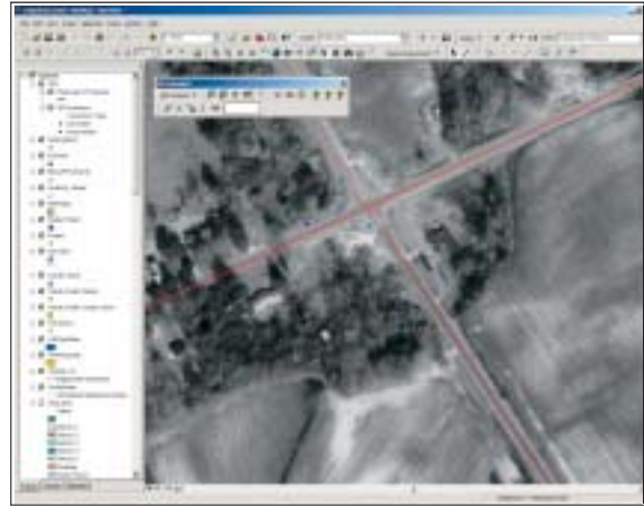
Overlaying corrected data on an orthophoto.
