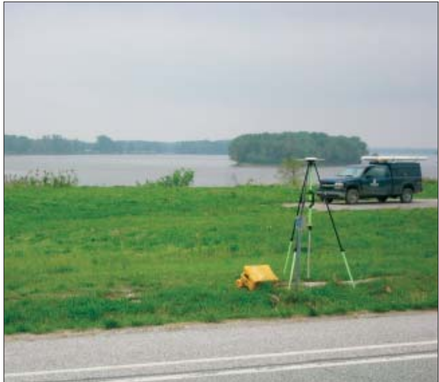
Woolpert surveying crew performing primary GPS observation on control along the Mississippi River.
