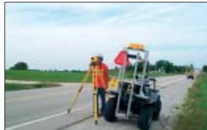
Geodetic leveling crews from the consultant using quad-runners while running leveling surveys.
