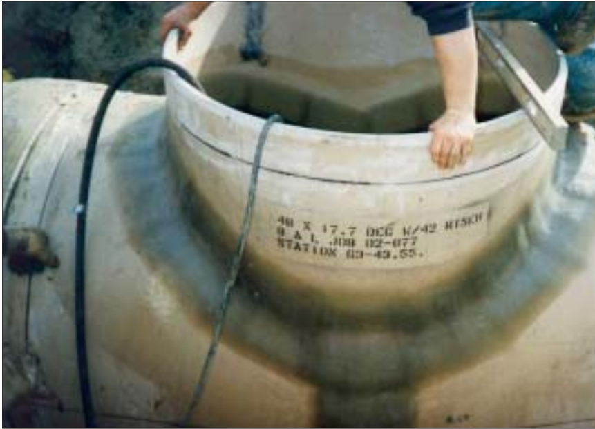
GRP manholes are made of centrifugally cast glass fiber reinforced unsaturated polyester resin. Joints between the individual manhole parts, such as concrete cones, pipe shafts, and base, have to be rendered watertight with bearing ring seals.
