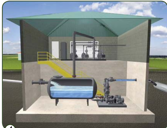
Vacuum stations are clean as well as operator friendly. Monitoring and maintenance are easy with a few gauges and charts checked daily and oil in the vacuum pumps changed regularly.
