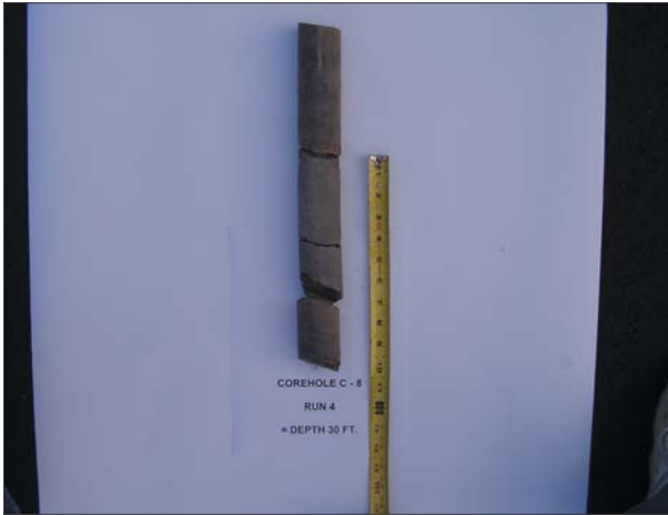
Grout column between intact rock layers.
