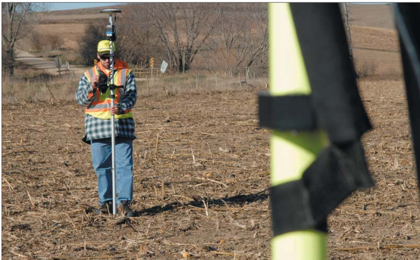
Only one field technician is required to collect real-time, centimeter-accurate survey points for a bridge replacement project.
