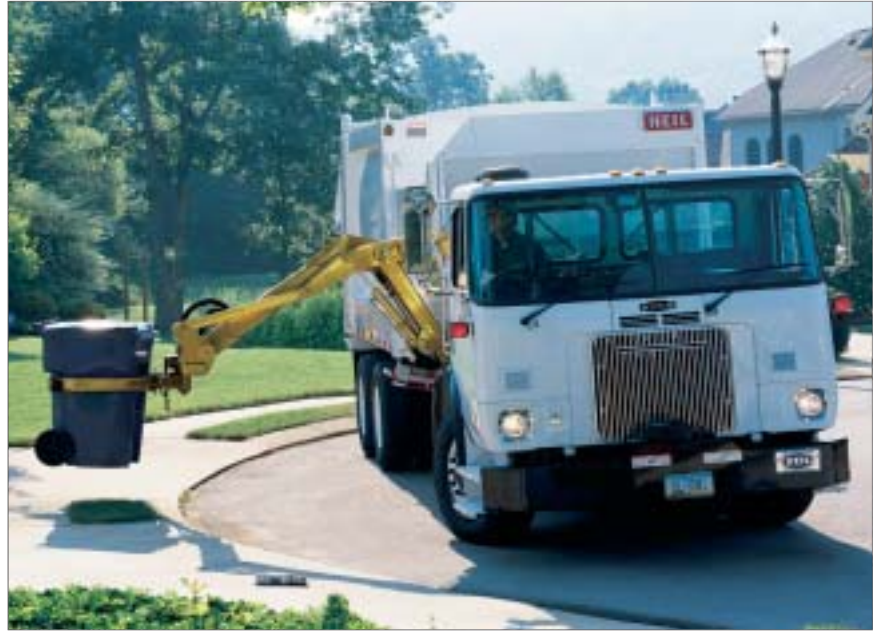
Operate-at-idle systems permit the refuse collection vehicle to lift and empty carts and compact refuse while the vehicle is at idle.
