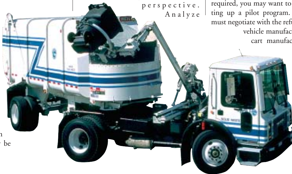
Heil's STARR™ System is a semi-trailer refuse collection system. When trailers become full they can be disconnected and the tractor hooked to an empty trailer so the operator can continue on his route. The trailer serves as a mini-transfers station; full trailers can be pulled as doubles to the landfill with non-route trucks.
