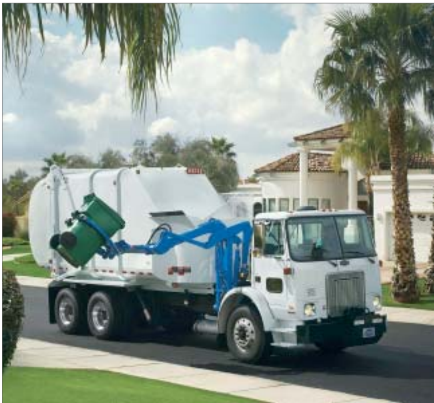
With automated refuse collection vehicles, the automated arm, truck body, and truck chassis are required to work together to be effective.
