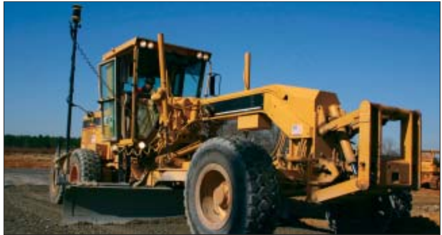
GPS-guided machine control systems automatically move the cutting edge of grading equipment to match the design grade.
