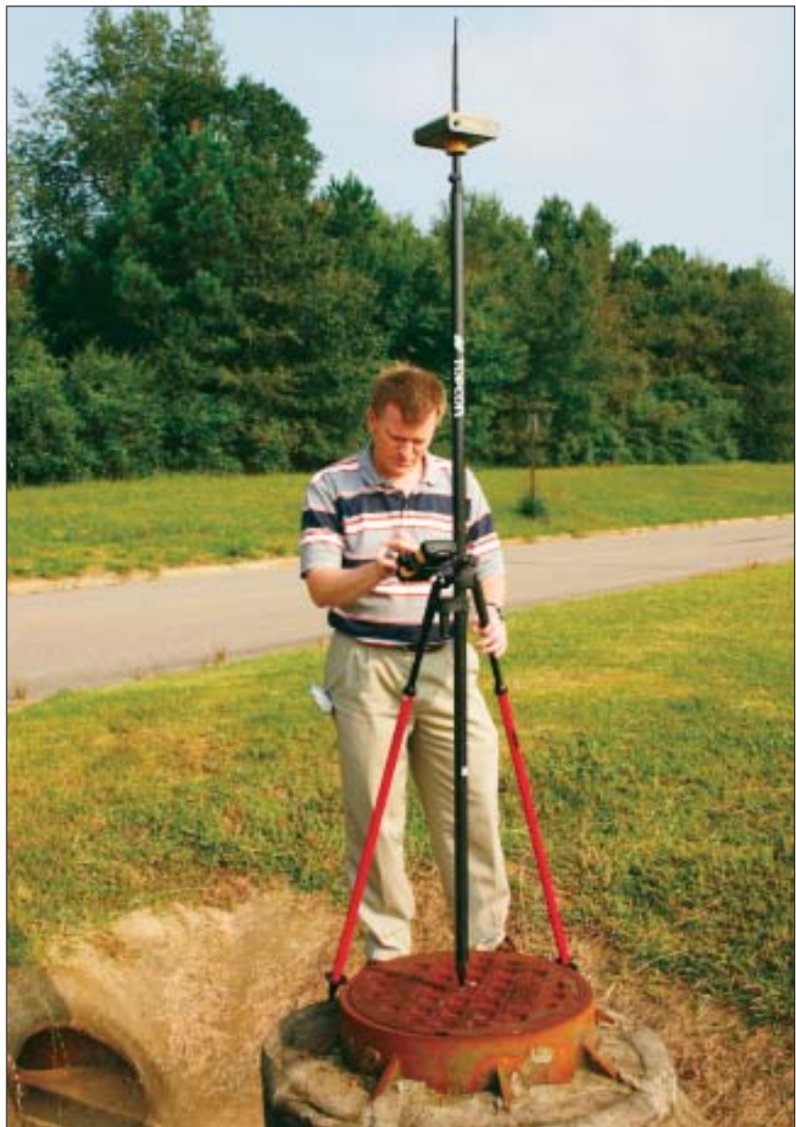
Topcon's HiPer Lite GPS survey system enable fast, accurate mapping of utility features for the GIS database.
