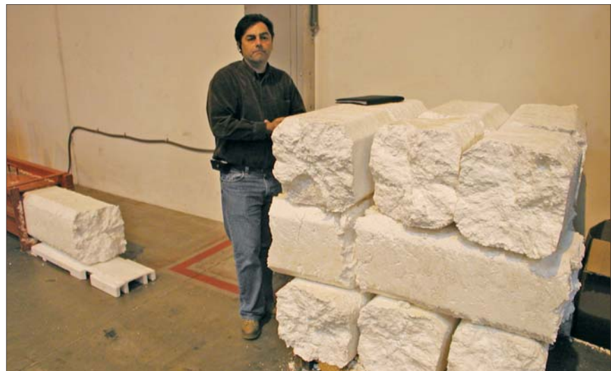
Compacted blocks are produced from the polystyrene at different rates by the three models of screw compactor available: 55 lb/hr, 250 lb/hr, and 500 lb/hr.
