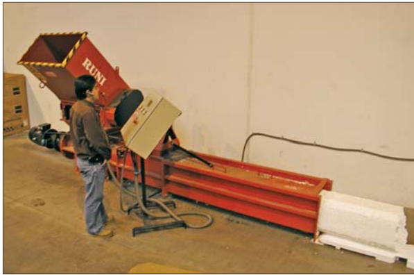
The screw compactor densifies the polystyrene with hydraulic, electronically-controlled jaws that maintain an almost constant compression pressure.
