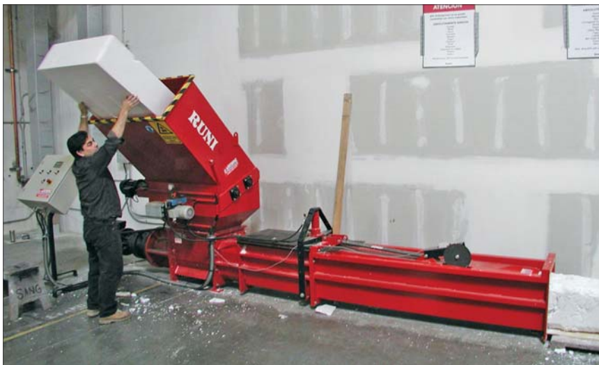
Polystyrene is manually fed into the feed hopper of the Runi screw compactor.
