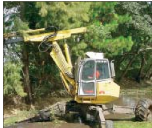
Menzi Muck mobile all-purpose excavators access tight areas where larger equipment dares not tread.
