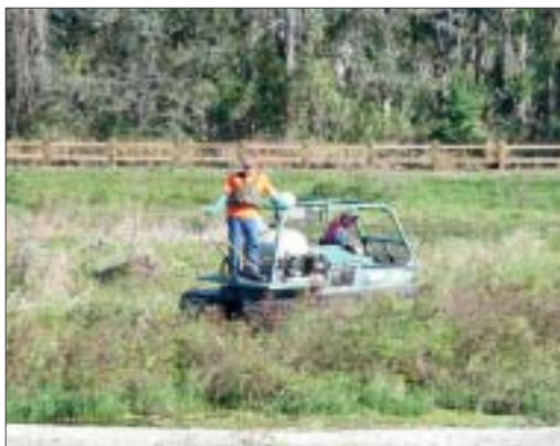
The Marsh Master can carry several men plus equipment over land, water, marsh, and swamp.
