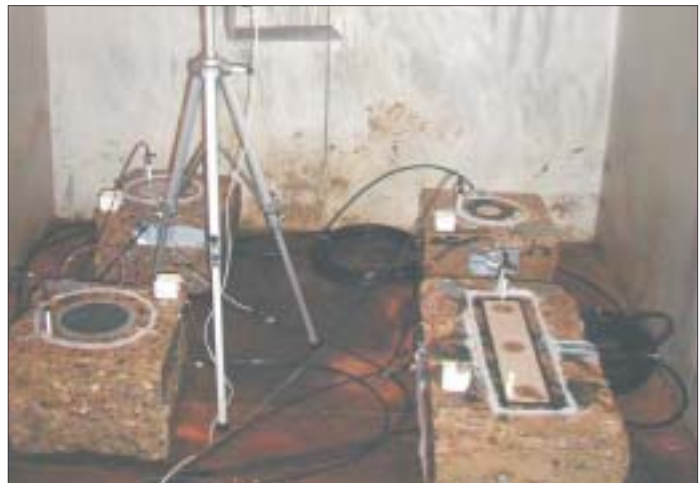
Top, an RWIS pavement sensor is installed in a cut slab of bridge deck for the bench test. At the upper left is an independent temperature probe. At the upper right and bottom center are thermistors attached to the block for additional independent temperature readings. At lower right is a Styrofoam block supporting another thermistor registering air temperature readings. The large circle was drawn around the sensor with silicone to confine the applied liquids. Not shown are the leveling screws mounted to the bottom of the block. Bottom, view of the entire experiment in the ORITE climate chamber with pavement sensors from three vendors installed in four blocks. The block shown in the top photograph is at the left front. The tripod holds a RoadWatch thermometer.
