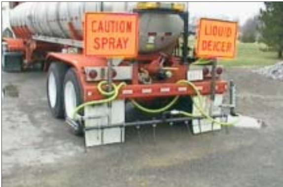
Top, application of brine pretreatment on road via a drip bar with ten outlets at the end of the truck. Bottom, Ohio Department of Transportation brine application truck.
