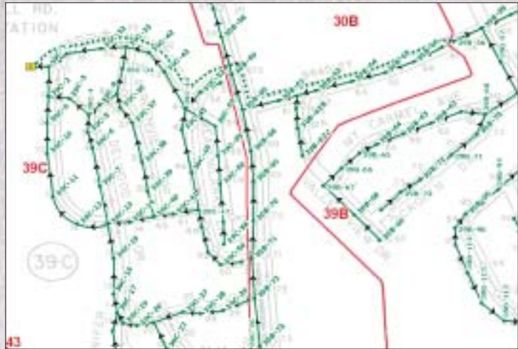
Overlay of scanned sewer maps and GIS layers depicting manholes with identification labels, pipes, flow direction, and sewer subareas.
