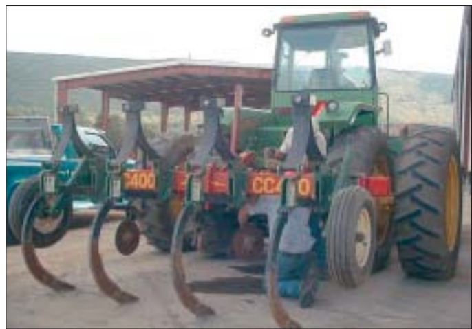
A sub-soiler, a tillage implement with few, stout, non-moving parts, is recommended for initial loosening of roadside sites. Roto-tillers are more suitable for incorporating topsoil or organic matter.
