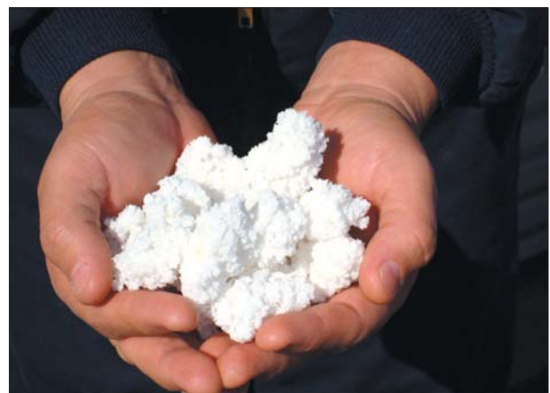
Smart Sponge is a polymer-based filtration material resembling popcorn, which absorbs hydrocarbons and other contaminants within its porous structure and has the capacity to destroy bacteria.
