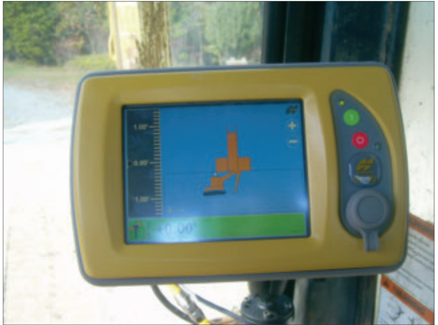
Mounted in the cab, the control box includes a monitor that helps the operator maneuver the bucket.
