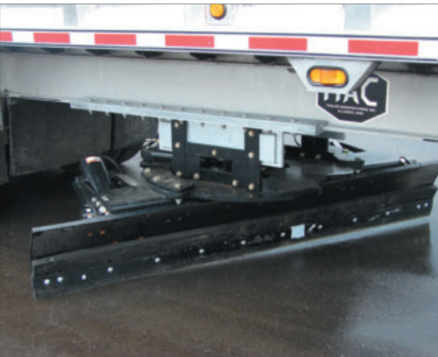
The trailer's ten-ft snowplow is centrally placed underneath the bed.
