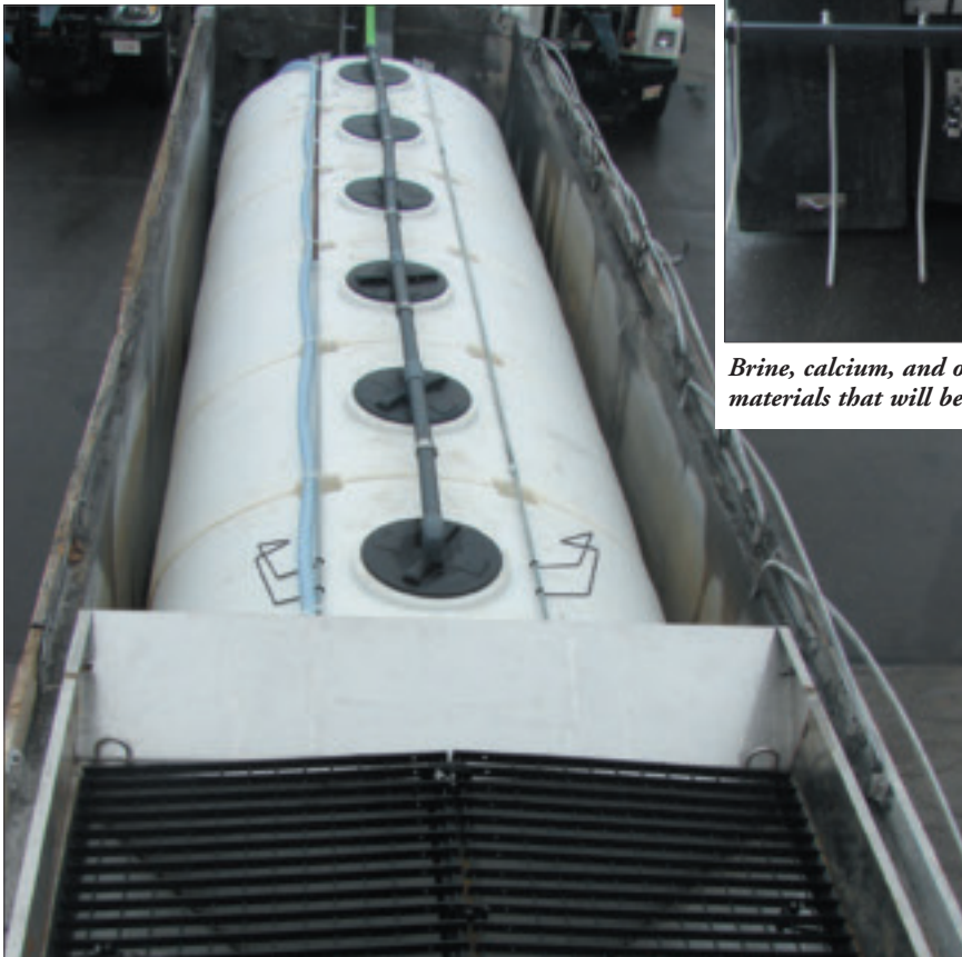
The multi-purpose trailer can hold 3,900 gal of liquid. The tank, shown here, actually consists of six, 650-gal tanks.
