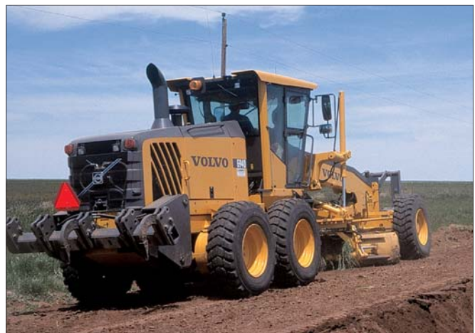
Nine motor graders are used in Deaf Smith County, TX, to remove large ruts from dirt roads and re-establish ditches after they have been beaten down by wind and rain.
