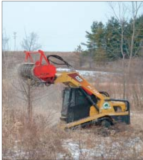
Mulcher allows operators to work their way into brushy areas from the top down.
