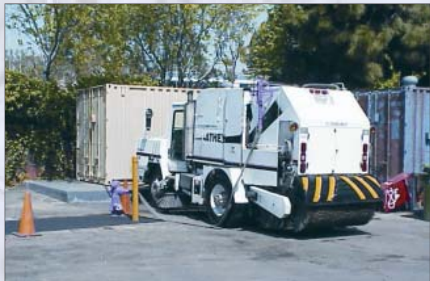
Sweepers and sewer flushers use the special recycled water hydrant to fill up with recycled water at the service center.
