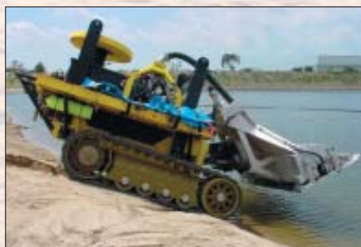
One of the basin cleaning vehicles (BCV) is for shallow lakes, where it is towed along the bottom by a cable system. Four are now in use.
