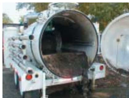
Pumper truck containing sediment sludge pumped from the swirl chamber.
