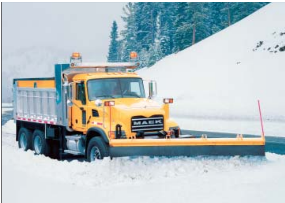
It is important for plowing crews to remove as much excess snow, slush, or ice before chemicals are applied to the road surface.
